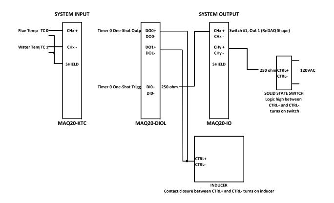
The alarm functions in the MAQ20-KTC module and the Special Functions of One-Shot Output and Trigger-to-Start in the MAQ20-DIOL Discrete Input / Output module enable the draft inducer to turn on at start of a burn and turn off on a differential temperature measured between two thermocouples.
